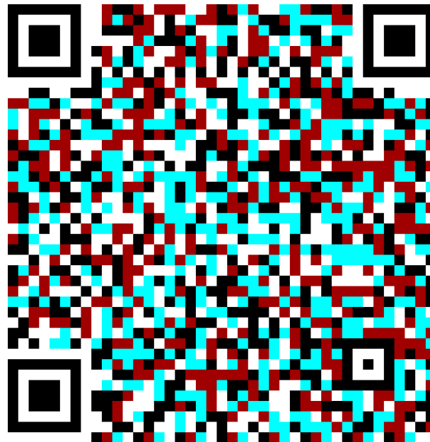
Figure 5.2: Example of a type 6H code using a four-color scheme (two bits per module).
