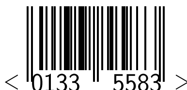
Figure 1.1: An example of an EAN-8 barcode.
