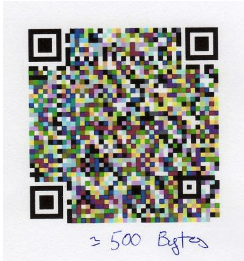
Figure 5.6: Successful desktop decoding of a sixteen-color symbol scanned with an Epson DX6000.
