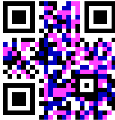
Figure 5.1: Example of a type 2H code using a four-color scheme (two bits per module) to represent data optically.
