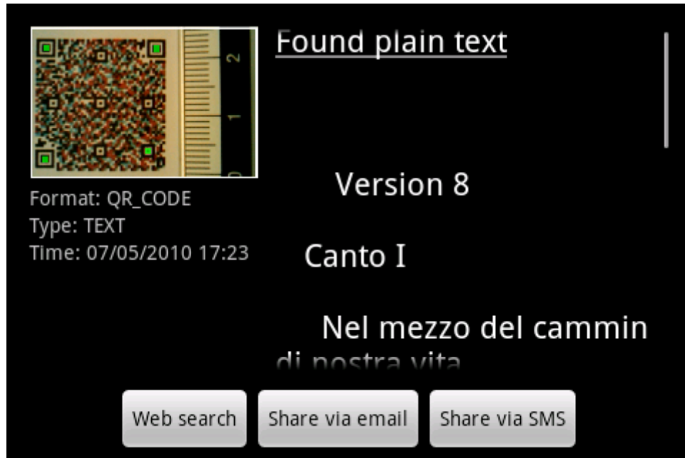
Figure 5.5: HTC Magic reading of a four-color Version 8L symbol measuring less than one square inch.
