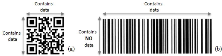
Fig. 1. Dimension for storing data in (a) 2D and (b) 1D codes.
